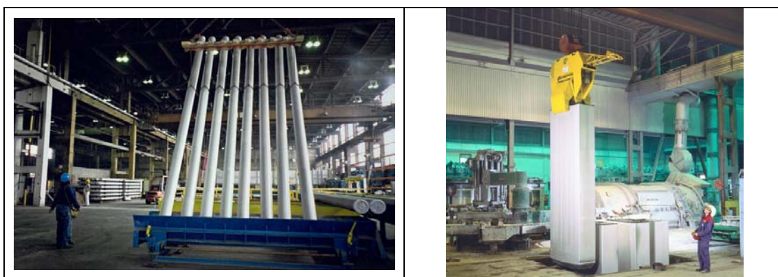
Fig. 3.3 DC-cast extrusion billets (cylindrical) or rolling slabs (rectangular)
